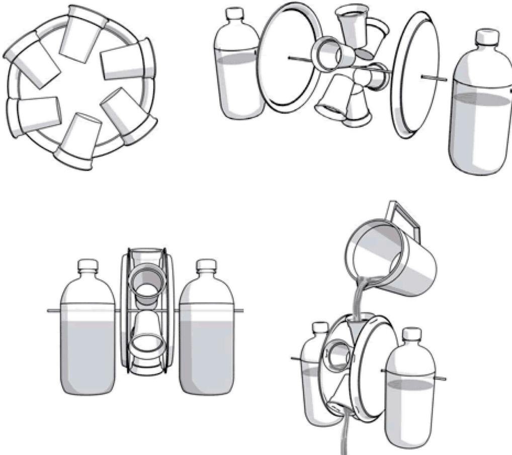
The wheel will need a hole in the centre for the axle to pass through and the buckets (*disposable cups*) will need to be arranged at equal distances around the edge of the wheel.
